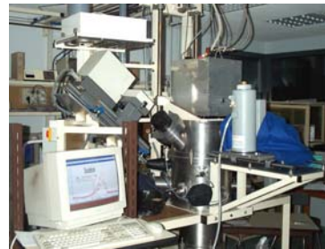
Set-up for measurement of luminescence stimulated by various in-situ excitation sources: electrical field, UV, temperature, plasma.
